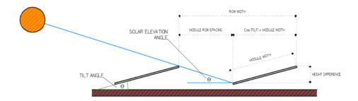
Height Difference = Sin (Tilt Angle) x Module Width
