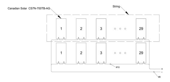
These two drawings give an idea into how the solar farm is laid out. It shows how the racks connect to the combiner box and then the combiners boxes go into the inverter. In the more detailed drawing, you can see how the panels are individually connected to make a string. You can also see the size of cable we will be using and the number of panels.
